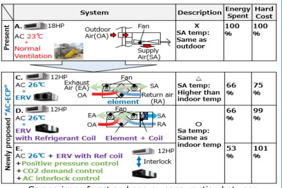
Comparison of cost and energy consumption between Present AC and AC-ECP
